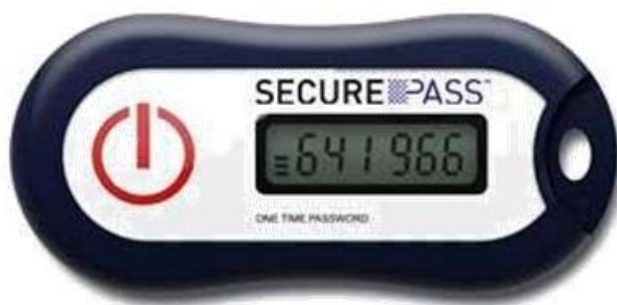
Fig. No. 2: A Time-synchronized Token by SecurePass
