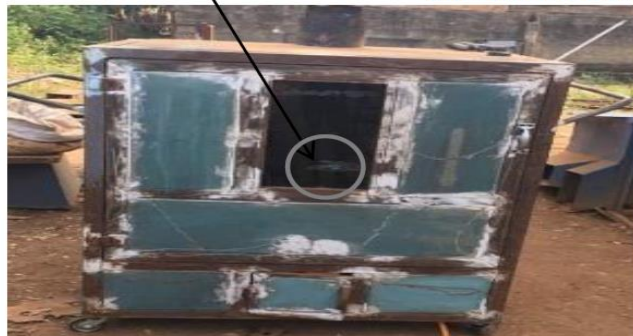
Figure 4a : Fabricated Gas oven
