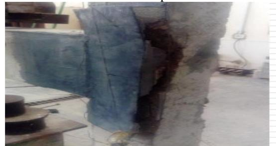
j- Failure condition of specimen S3-700.
