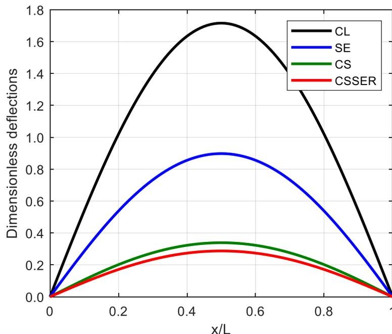
**Fig. 2 Dimensionless deflections of simply supported FGM Timoshenko nanobeam for different analyses (CL, CS, SE and SEER) at ( $k = 1, h = 5\text{ nm}, b = h, L = 15h, l = h$ ).**
