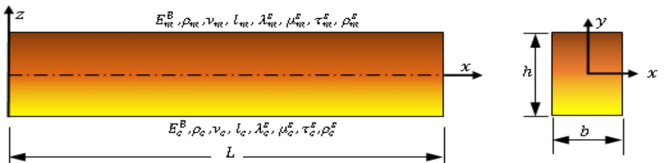
**Fig. 1 Schematic of a functionally graded nanobeam with surface layer.**
