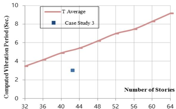
Fig. 25 Average Values of Vibration Periods in- for Tube-in-Tube of Fig. 3.
