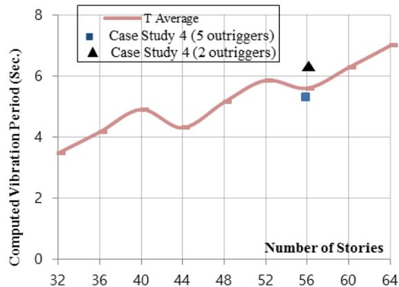
Fig. 32 Average Values for Vibration Tube-in-Tube of Period for Tube-in-Tube of Fig. 4.
