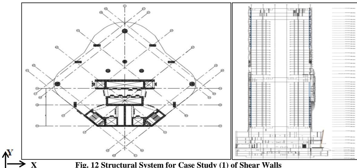
Fig. 12 Structural System for Case Study (1) of Shear Walls
