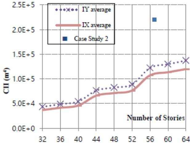
Fig. 13 Average Values for CII for Shear Walls of Fig. 2.
