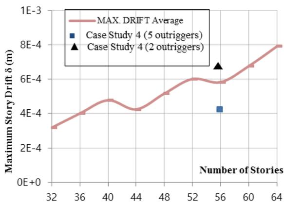
Fig. 31 Average Values for Maximum Drifts for Fig. 4.
