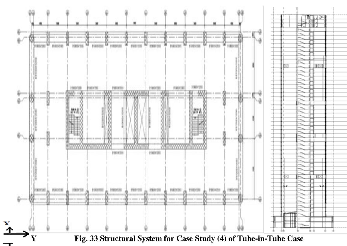
**Fig. 33 Structural System for Case Study (4) of Tube-in-Tube Case**
