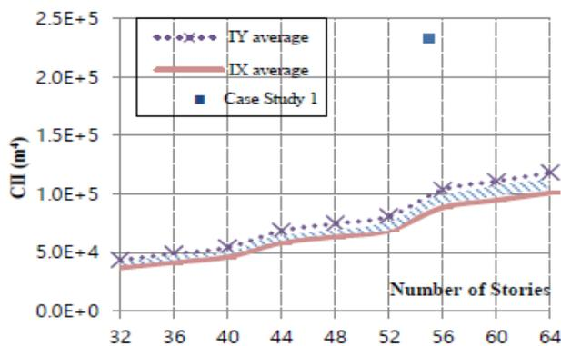
Fig. 6 Average Values CII for Shear Walls of Fig. 1.
