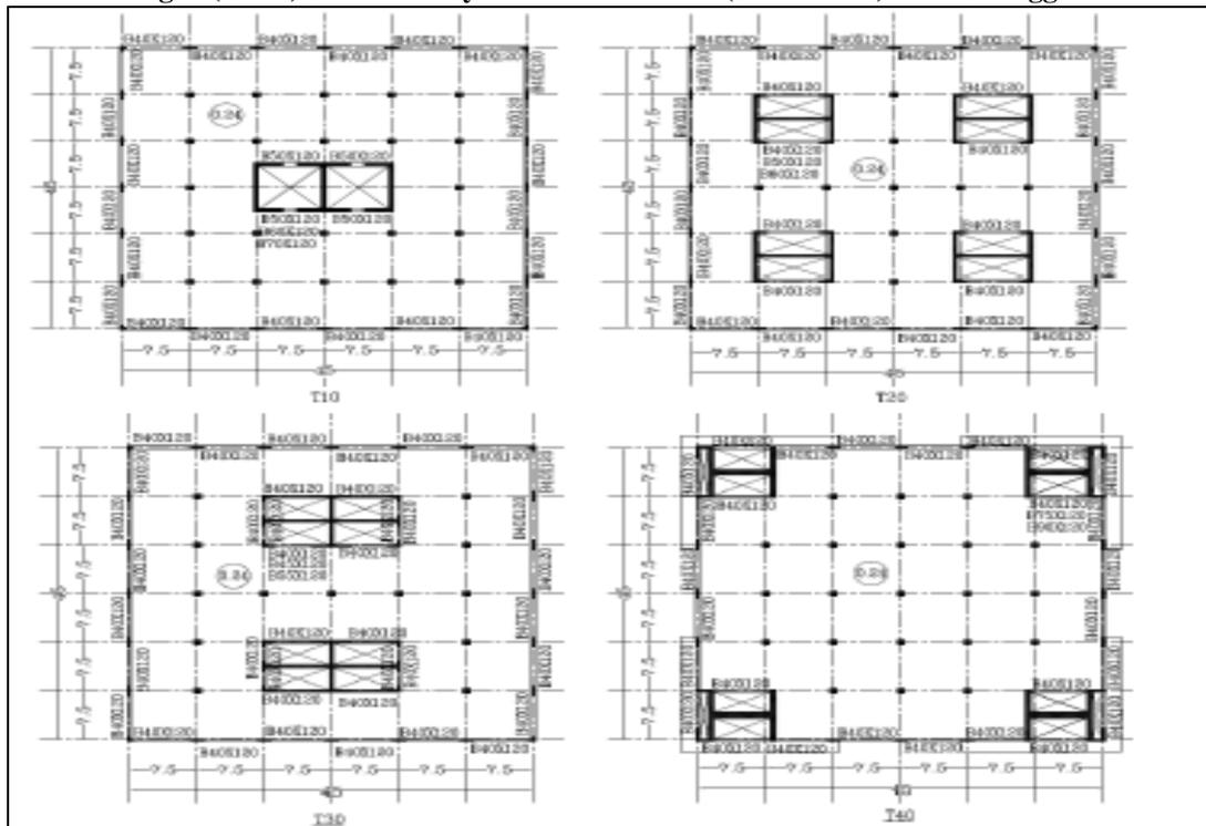
Fig. 3 Structural Systems used in Tube-in-Tube.
