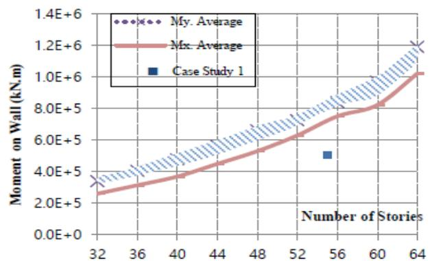
Fig. 7 Average Moments for Shear Walls of Fig. 1.
