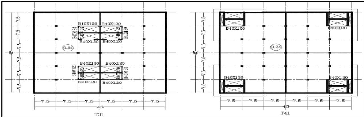
Fig. 4 (Cont.) Structural Systems used in Tube-in-Tube with Outrigger.
