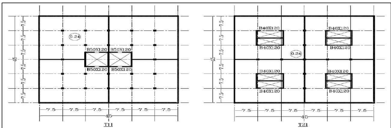
Fig. 4 Structural Systems used in Tube-in-Tube with Outrigger.
