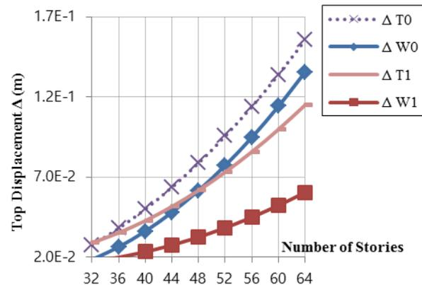
Fig. 37 Comparing Top Displacement averages for all 4 systems.
