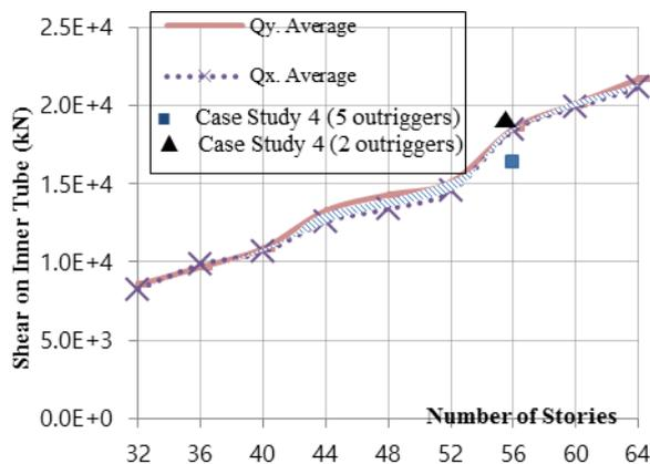
Fig. 29 Average Values of Shear Forces on Inner Tube for in-Tube of Fig. 4.
