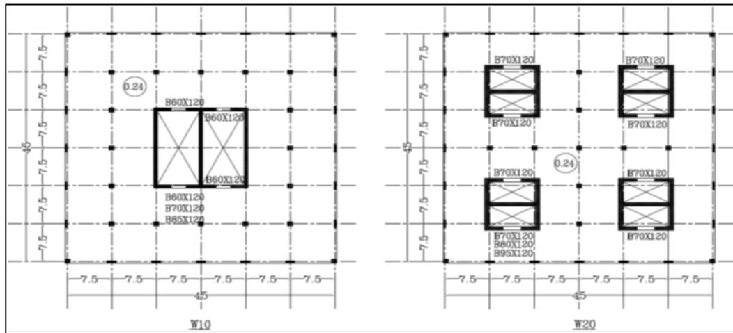
Fig. 1 Structural Systems used in Core (Shear Wall) Case.
