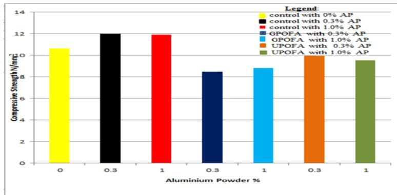
Figure 4.3: Compressive Strength and Aluminum Content after 28 days
