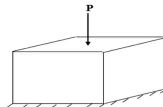
Figure 3.2: Compressive Test Specimen
