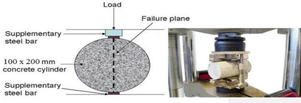
Figure 3.3: Splitting Tensile Specimen and Test Machine
