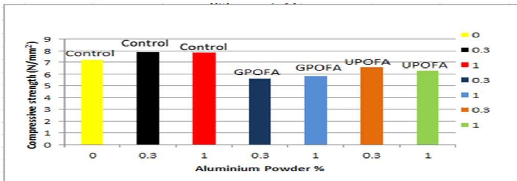
**Figure 4.1: Compressive Strength and Aluminum Content after 7 days**
