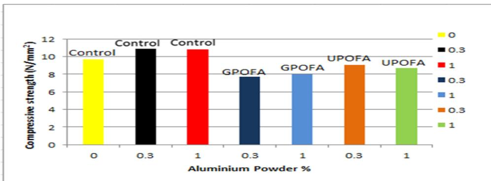
Figure 4.2: Compressive Strength VS Aluminium Content after 14 days
