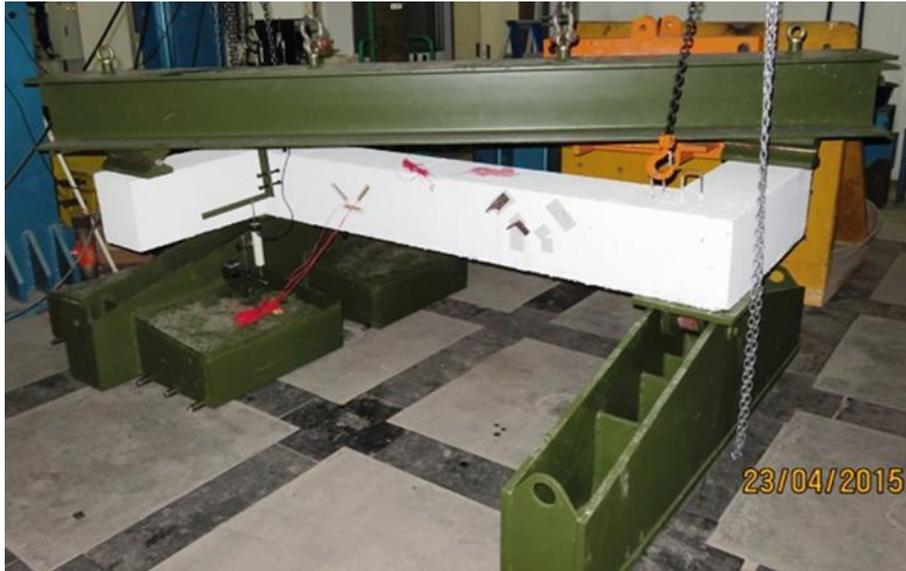
Figure 5. Experimental setup of the beam
