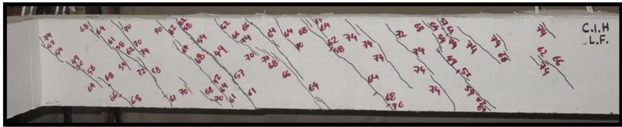
Figure 15. Crack patterns of beam C-1-H
