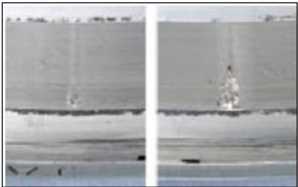
c. Pitting on the outer ring 2-row cylindrical roller bearings
