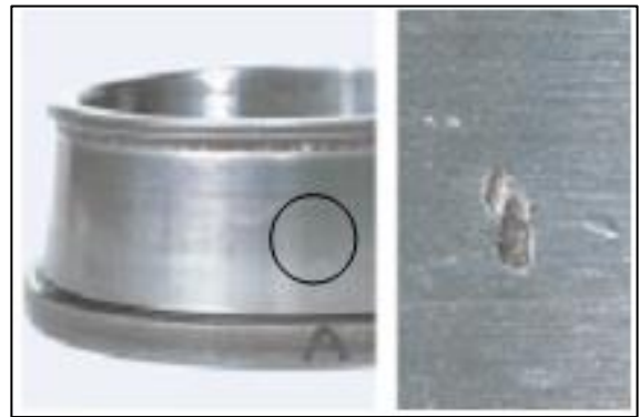
d. Pitting on the ring in a taper roller bearing
