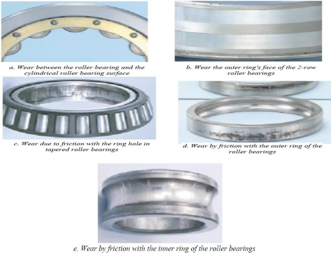
Figure 6. Some pictures of wear of the bearings
