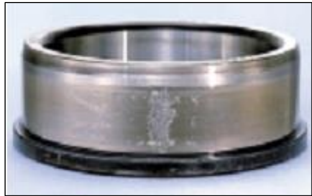
b. Pitting on the inner rings in cylindrical ball bearings
