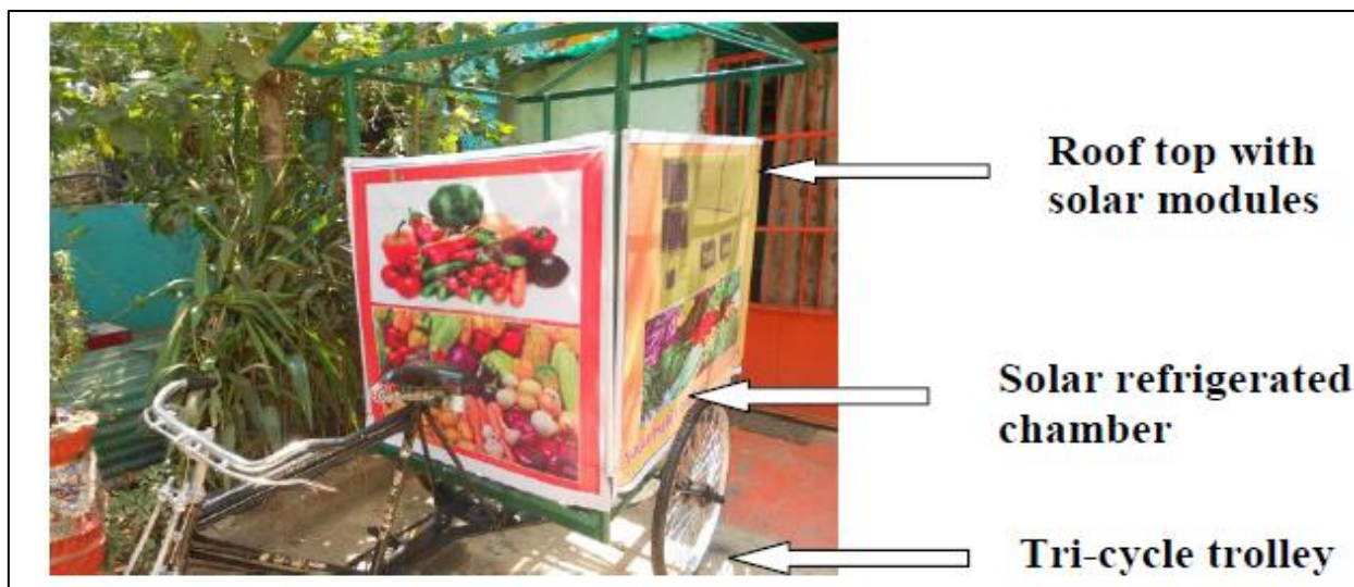
Solar Refrigerator Mounted on Tri-cycle
