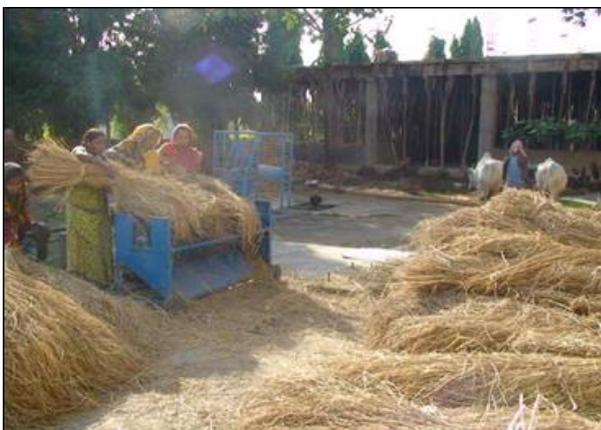
Fig.2 Multi crop thresher cum winnower used in rotary mode
