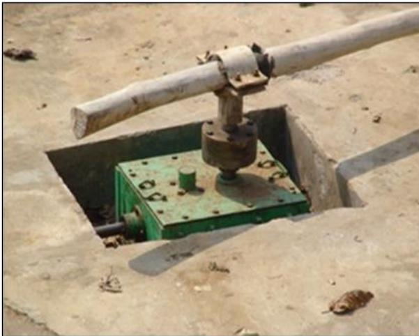
Fig.1 Gear box unit for mechanical power in rotary mode
