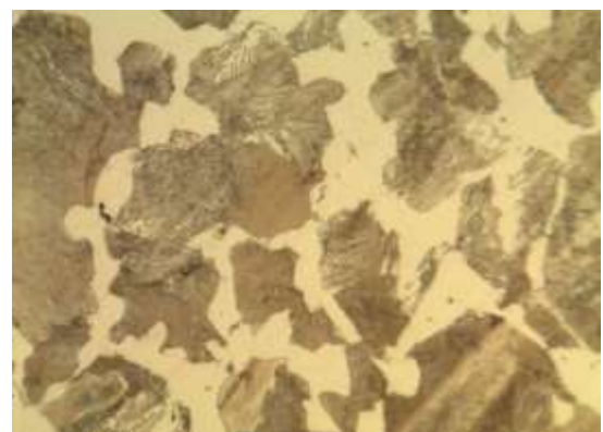
Fig-12: Untreated/As casted microstructure feature of CSN 12050 carbon steel 500x
