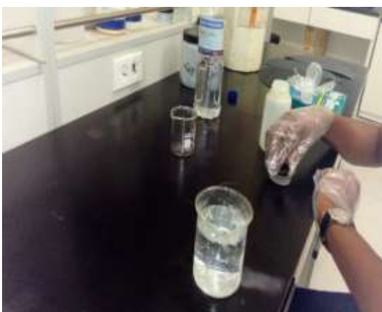
Fig-6: Etching (methyl and nitric acid)
