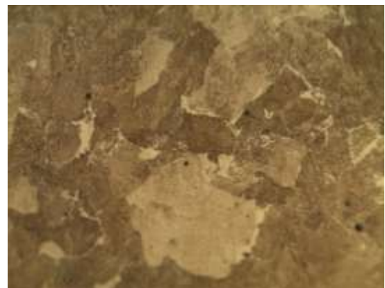
Fig-11: Tempered microstructure feature of CSN 12050 carbon steel 500x
