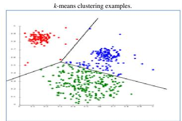
Fig-2: Voronoi cells partitioned by k-means algorithm (Färber, et al., 2010)
