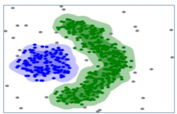
Fig-11: Density-based clustering with DBSCAN (Goebel, 2014).
