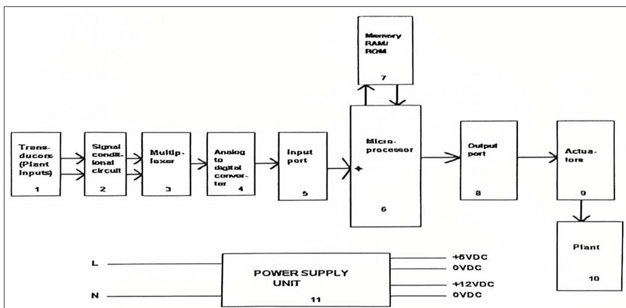
Figure 3: Detailed system block diagram
