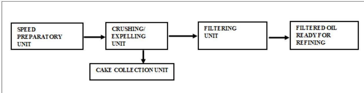
**Figure 1: Existing physical system of groundnut oil Extraction System**
