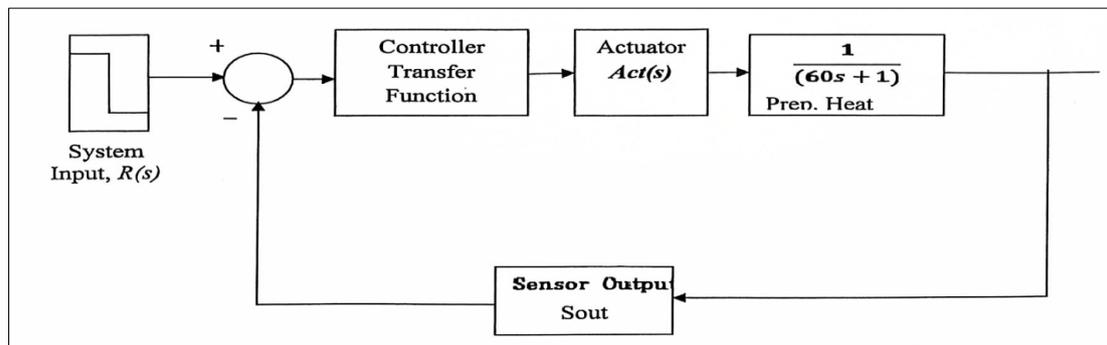
**Figure 4: Block Diagram of the Closed Loop Temperature Control System**
