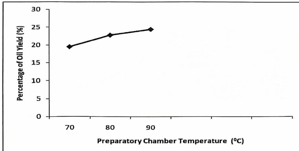
**Figure 7: Graph of percentage of oil yield against preparatory Chamber Temperature for the stabilized chamber**
