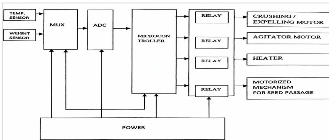
Figure 2: Block Diagram of the Proposed Groundnut Extraction System
