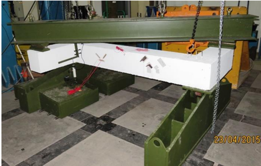
Figure 5. Experimental setup of the beam
