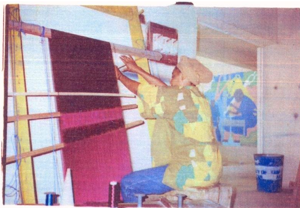
The warping process on the vertical loom (rolling thread on the loom) in Kogi Central
