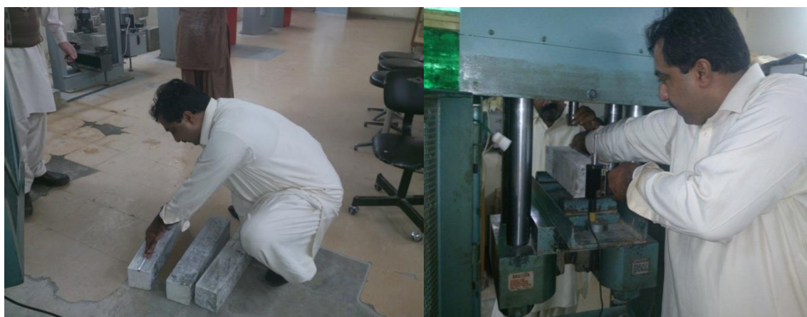
Figure 3 & 4 shows size of beams checked and Placing of Beams in Universal Testing Machine.
