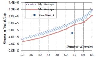
Fig. 7 Average Moments for Shear Walls of Fig. 1. shear walls and displacements of building are presented
