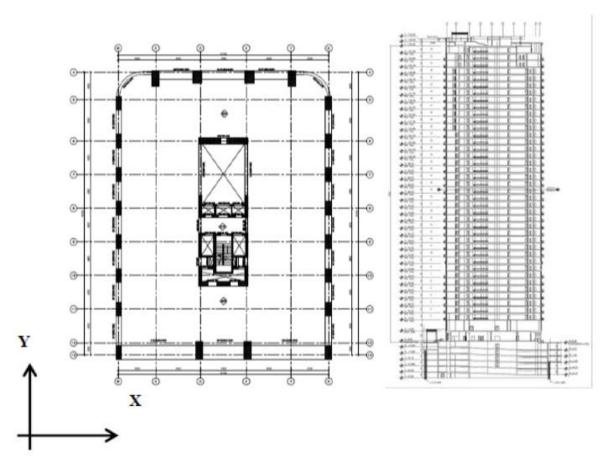
Fig. 26 Structural System for Case Study (3) of Tube-in-Tube Case
