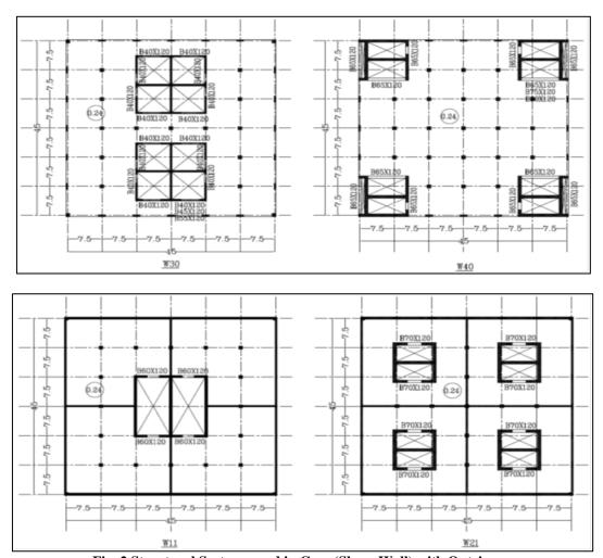
Fig. 2 Structural Systems used in Core (Shear Wall) with Outrigger.
