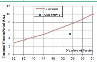
Fig. 11 Average Values for Vibration Periods for Shear Walls of Fig 1
