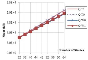
Fig. 36 Comparing Shear Force averages for systems.
