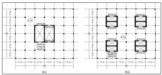
Fig. 1 Structural Systems used in Core (Shear Wall) Case.
