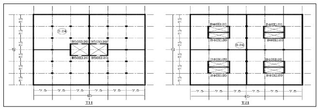
Fig. 4 Structural Systems used in Tube-in-Tube with Outrigger.
