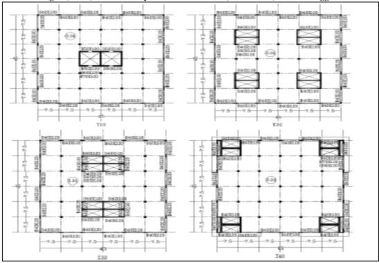
Fig. 3 Structural Systems used in Tube-in-Tube.
