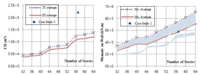
Fig. 13 Average Values for CII for Shear Walls of Fig. 2. Fig. 14 Average Values for Moments for Shear Walls of Fig. 2.
