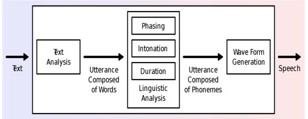
Fig 2: Overview of a typical TTS system (*Wikipedia*)
