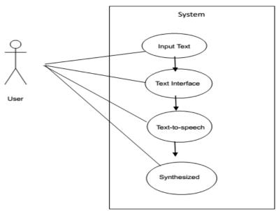
Fig 5. Use case diagram for the voice synthesizer
