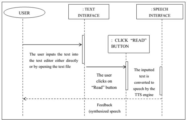
Fig 6. Sequence diagram for the TTS voice synthesizer
