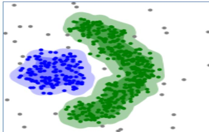
**Fig-11: Density-based clustering with DBSCAN (Goebel, 2014).**
