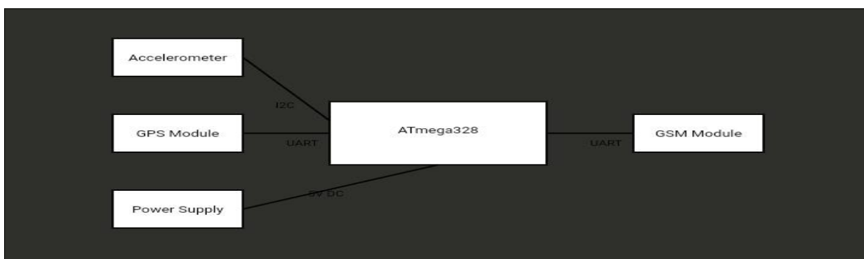
Figure 3: Circuit Layout Diagram (Diagram of the hardware configuration in IVADS)
