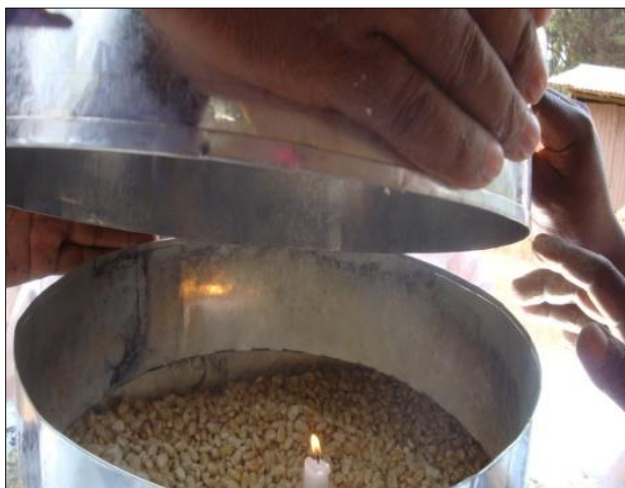
Figure 1: Candle light over the grain of loaded metal silo for oxygen depletion
